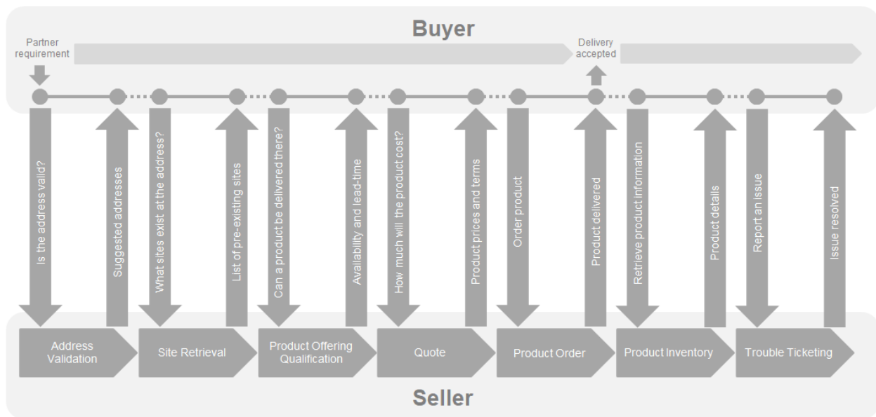
Figure A1-1 – Cantata and Sonata End-to-End Function Flow
